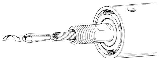
Slide the wedge over the core (7 strands) of the wire .
