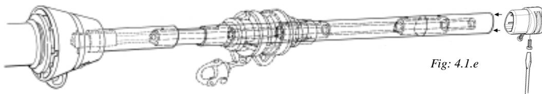
Fit the halyard swivel over the top end of the extrusion, slide it down as far as the sail feeder gap and secure it in this position with adhesive tape. Fit the top guard and secure it with the two pre-fitted screws. Tighten the screws until they bottom, but do not over-tighten.
