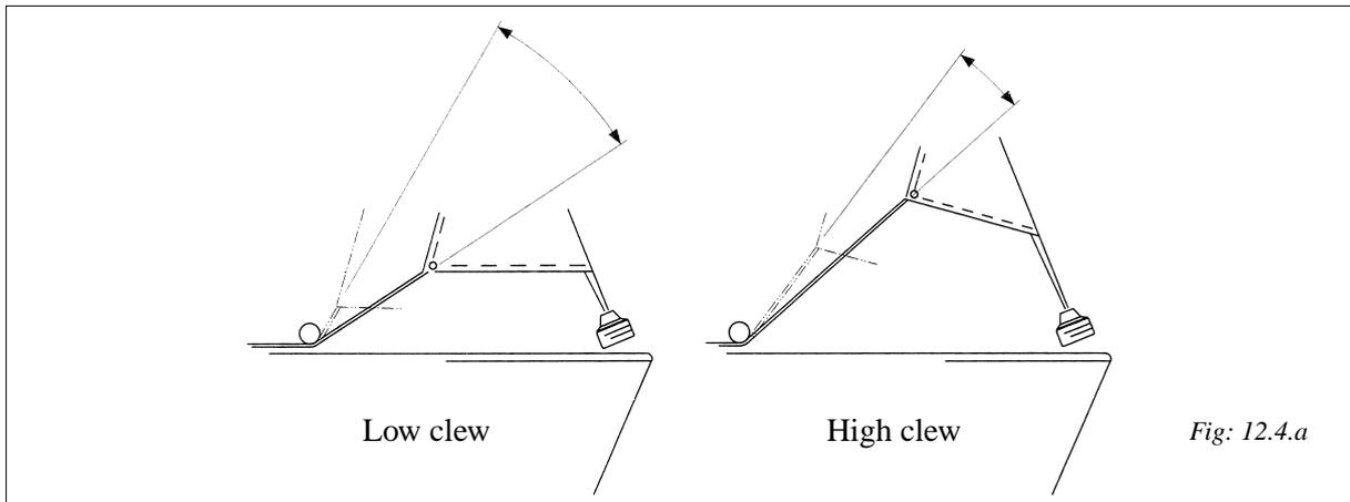
The angular variation of the sheet relative to the deck is less for a high-clew sail. The comparison is based on the same number of furling revolutions.
