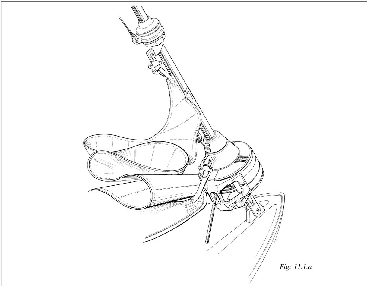
5. Attach the sheet to the clew. Take the sheet through the lead block and then on to the cockpit. Put a figure-of-eight knot in the ends.
