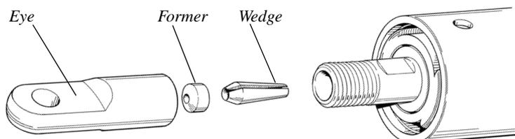
Unscrew the eye, wedge and former from the terminal part.
